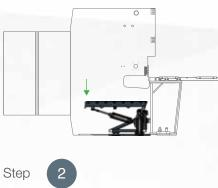
Once the cutting process is kicked off, the table comes down lower position at the same time and this will ensure cutting sheets placed over the table again as seen in the picture. DURMA IV
