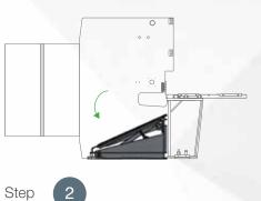
Once the cutting process is kicked off, the table comes down lower position at the same time and this will ensure cutting sheets placed over the table
