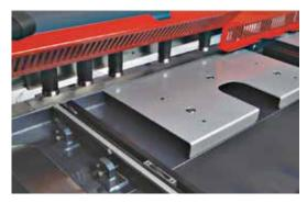
Flip-up Finger Guard Adjustable Ball Transfer Table Hydraulic Holddowns
