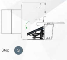
After cutting process is finished, sheets are discharged by closing movement of the table.
