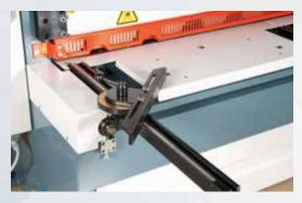
Adjustable Angle Stop 0-180° Finger Guard Ball Transfer Table Hold Downs with Rubber
