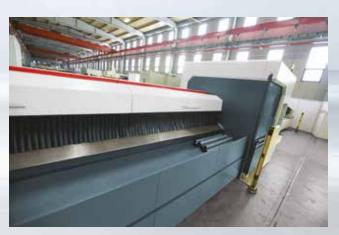
For longer parts than 800 mm, unloading table enters the cabin and unloads the parts.
