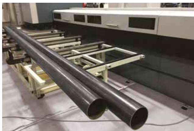
Tubes up to 6 m of length are removed by automatic unloading system with conveyor.
