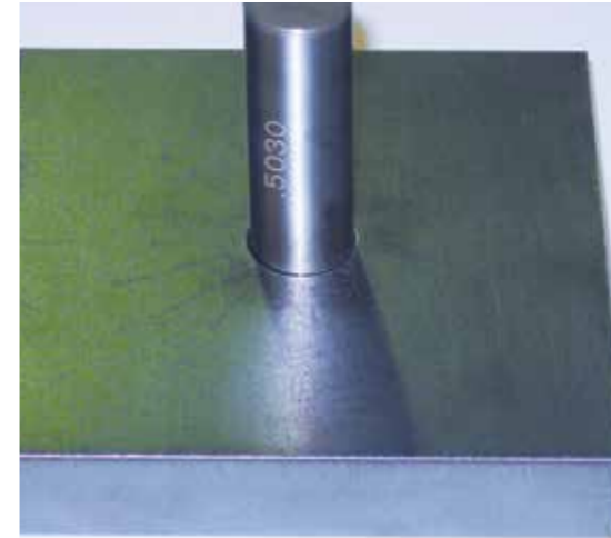
With True Hole technology cut with HPRXD Plasma
