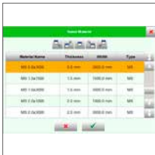
Automatic material sheet thickness adjustment, controlled by ProLink S
