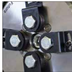
Automatic locking of Combi clamping beam.
