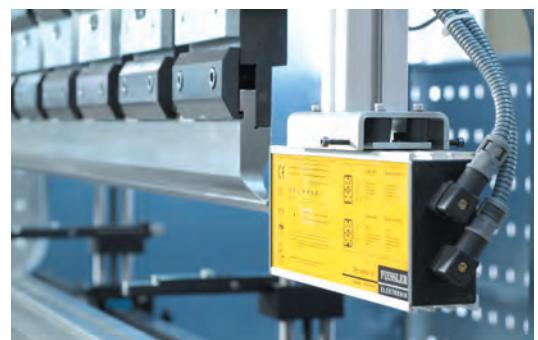
Ce Laser Safety System
